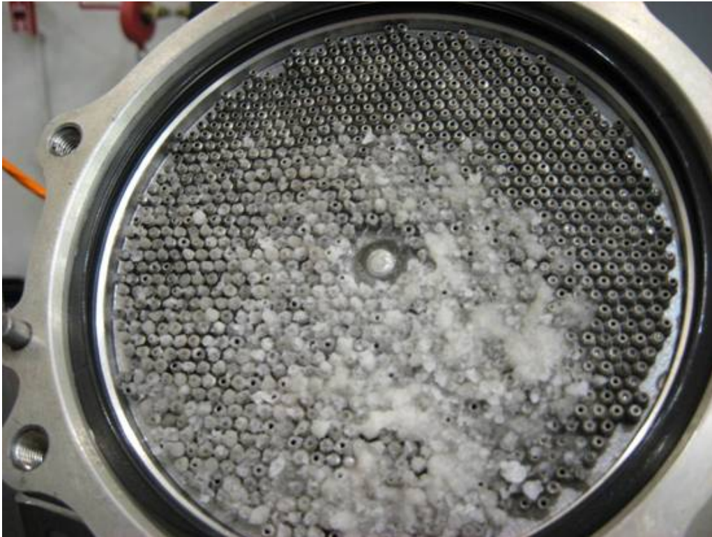
Figure. Ice on the inlet face of a Rolls-Royce RB211 Trent 800 series FOHE.
