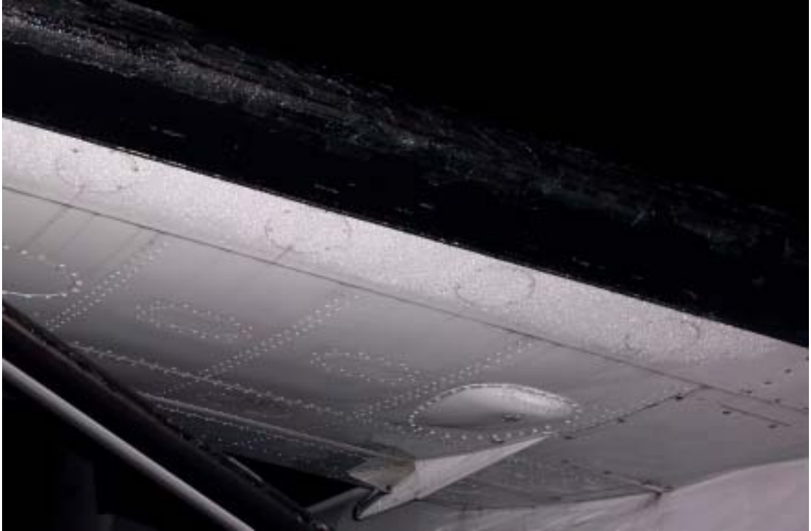
Figure 2. Photograph of the right wing lower surface, showing ice accumulation aft of the leading edge deice boot.
