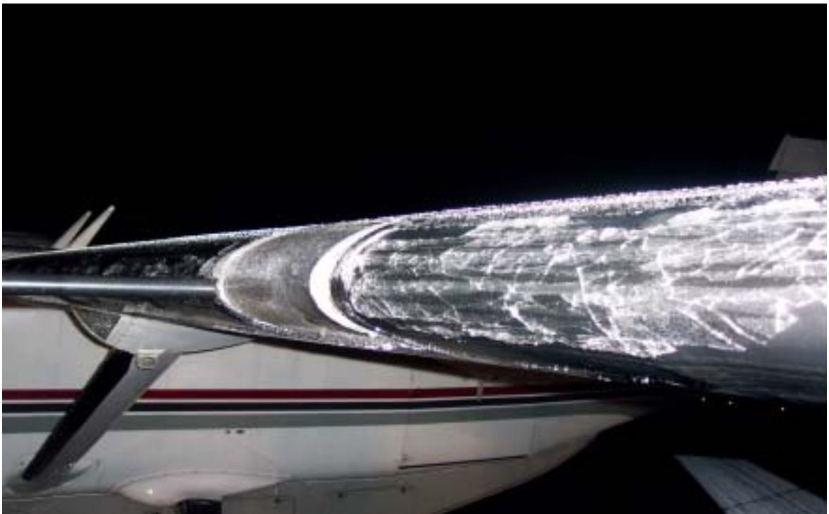
Figure 1. Photograph of the left wing leading edge, showing ice accumulation aft of the deice boot.
