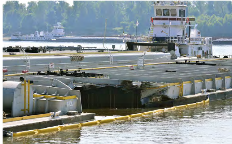
Figure 17: Damaged barge APEX 3508 from Dewey R tow; shell and deck plate have been removed. PHOTO BY COAST GUARD
