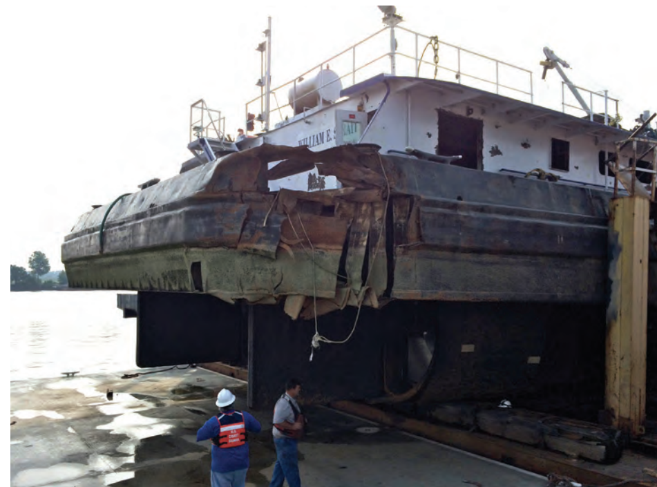
Figure 35: Damaged hull near the starboard stern of the towing vessel William E Strait . Photo taken after the vessel was salvaged.
