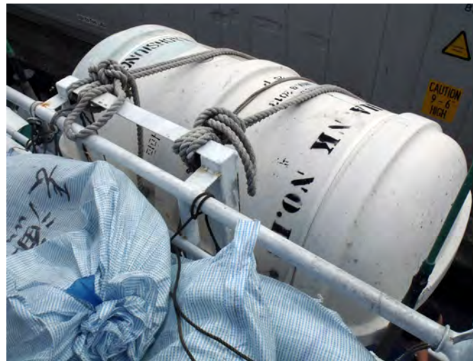
Figure 59: Liferaft aboard sister-vessel SeaHawk No. 18 secured to its cradle with lines. PHOTO BY COAST GUARD
