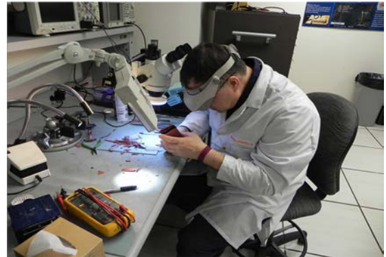
Figure 8 A flight data recorder being disassembled and inspected by an NTSB engineer from the Office of Research and Engineering at the NTSB laboratory in Washington, DC.
