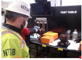
**Figure 13** An NTSB materials engineer cuts a section of pipe for the investigation of a crude oil leak from a subsea pipeline crack that occurred in Newport Beach, California, on October 1, 2021. The NTSB released DCA22FM001 for the public docket on March 31, 2023.
