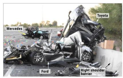
**Figure 7** At-rest position of the multivehicle crash that occurred in Phoenix, Arizona, June 9, 2021. A commercial truck traveling eastbound on SR-202 crashed into a queue of passenger vehicles that were stopped because of road closure. The NTSB issued Highway Investigation Report 23/04 on March 28, 2023, detailing our investigation of the crash. (Source: Arizona Department of Public Safety, with annotations by the NTSB).
