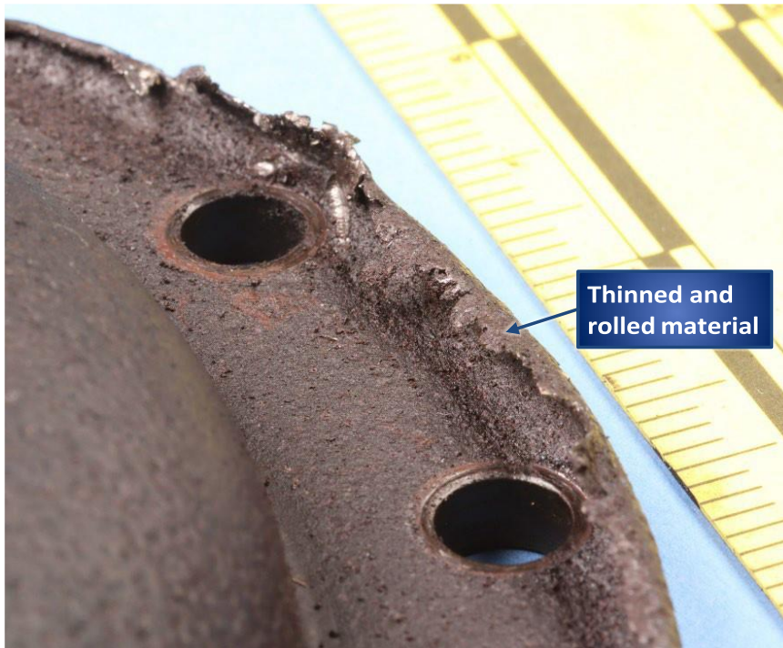
Figure 7. Outer flange separation surface at the outside diameter of the rear bearing cover.
