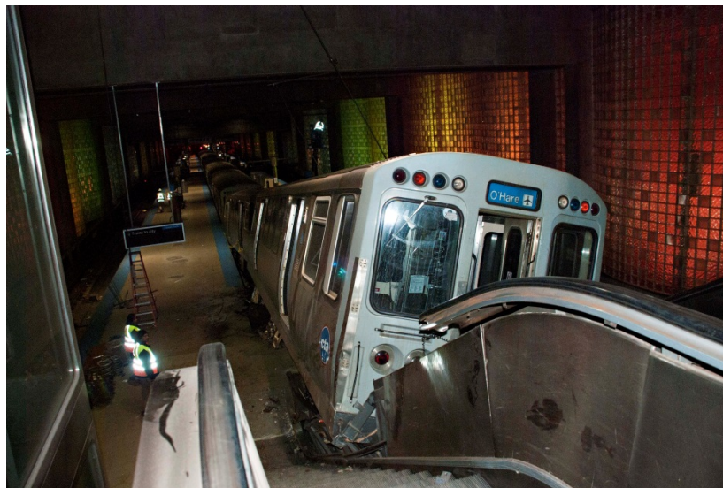
Figure 1. View of derailed train car that struck the escalator.
