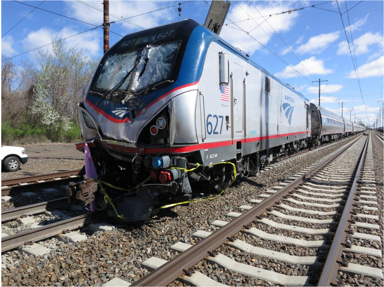
Figure 1. Damage to Amtrak passenger train 89.
