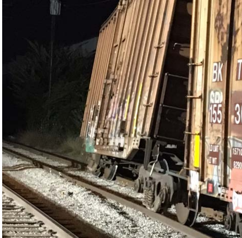
Figure 1. Photo of derailed boxcar.
