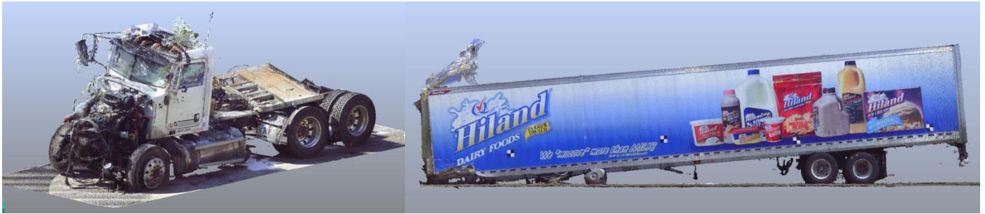
Figure 1. Image from 3D scans of the 2013 Peterbilt truck-tractor and 2014 Great Dane semitrailer combination vehicle.
