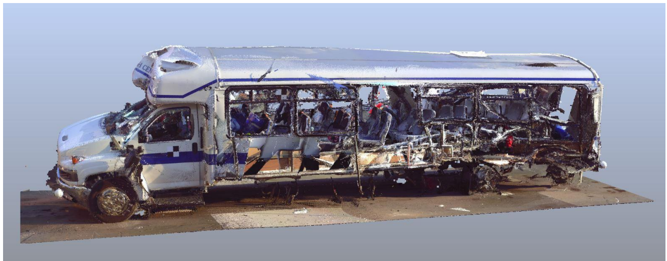
Figure 2. Image from 3D scan of the 2007 Chevrolet C5500 / 2008 Champion 32-passenger medium-size bus.
