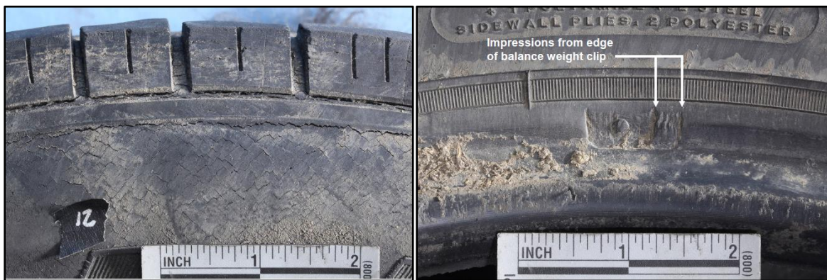
Figure 7. At left, cracking on inboard sidewall. At right, impressions left by balance weight clip.
