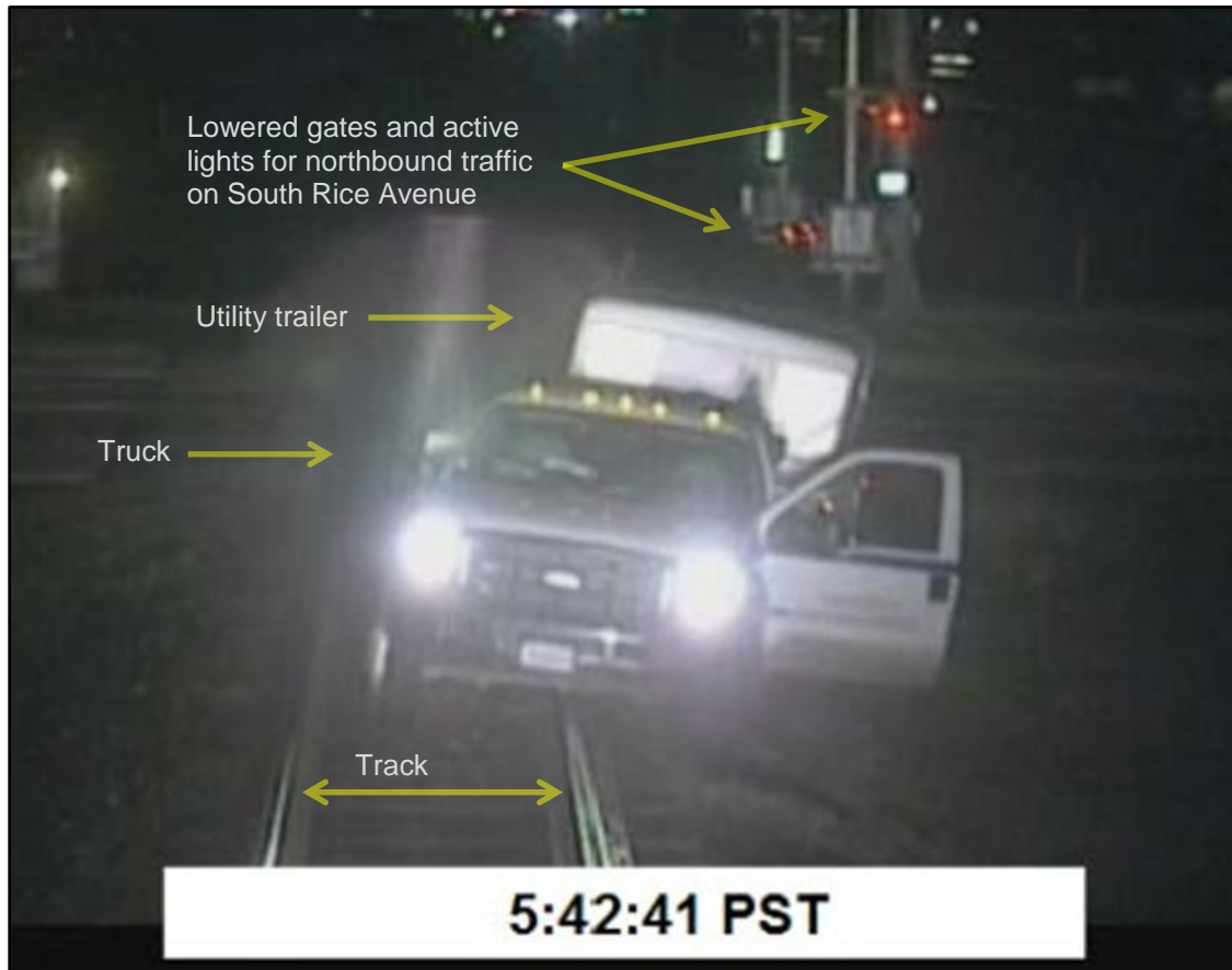
Figure 5. Still image from train's forward video camera, showing disabled truck straddling south rail, with headlights on and driver door open; utility trailer behind the truck; and South Rice Avenue grade crossing in background, with its gates down and lights active.
