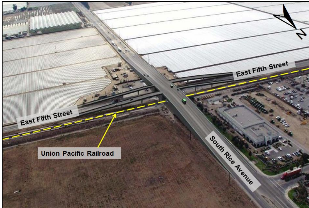
Figure 10. Conceptual representation of future grade separation of South Rice Avenue over UP track and East Fifth Street.
