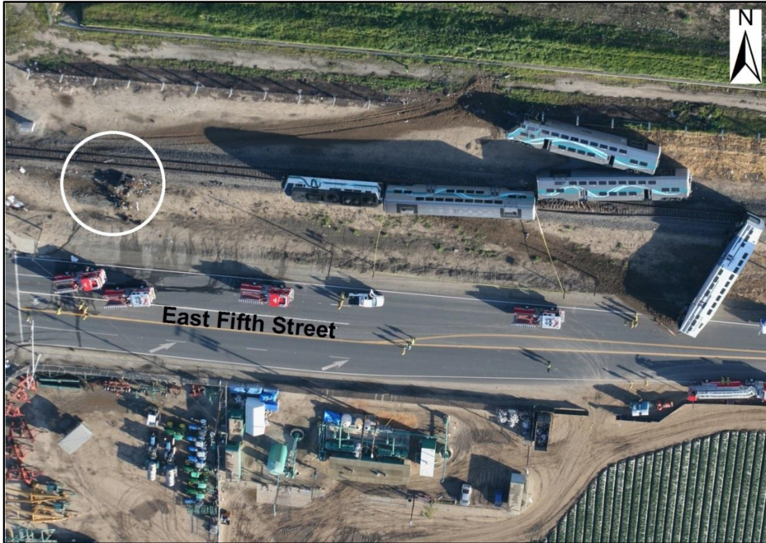
Figure 2. Northward-facing aerial view of train at final rest, showing (a) rear locomotive; (b) three overturned railcars and one derailed but upright railcar, with railcar at far right blocking part of East Fifth Street; and (c) remains of truck circled at left.
