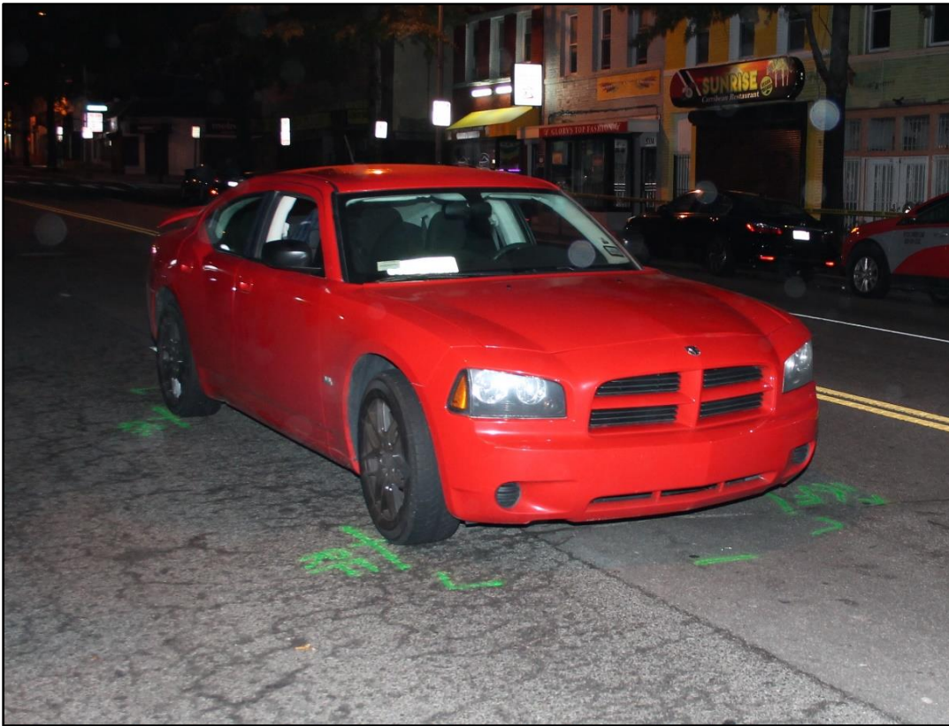
Figure 3. Crash car photographed at final rest position on Georgia Avenue NW. Green marks on pavement preserve position of wheels for investigative purposes.
