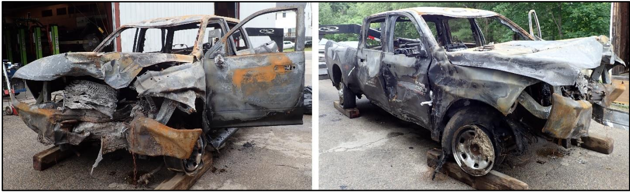
Figure 6. The pickup truck postcrash, with damage to the front end (left) and the right side (right).
