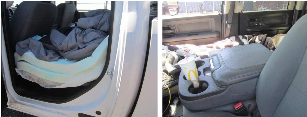
Figure 9. Exemplar vehicles from Westfield Transport with noncompliant sleeper berth, showing bedding placed across the rear seats (left image), and across the front passenger and rear passenger-side seats (right image).
