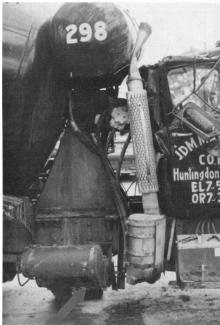
Figure 4 -- Location of missing drain valve indicated by arrow.
