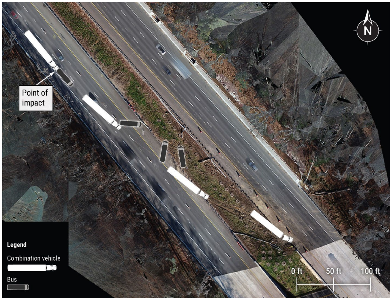
Figure 3. Depiction of the postimpact paths of travel for the truck and bus relative to physical evidence as overlaid atop the scene (orthomosaic image).
