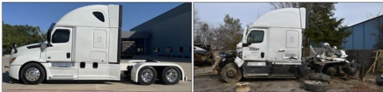
Figure 6. Exemplar truck-tractor (left; source: Vanguard Truck Center). Crash-damaged truck-tractor (right).
