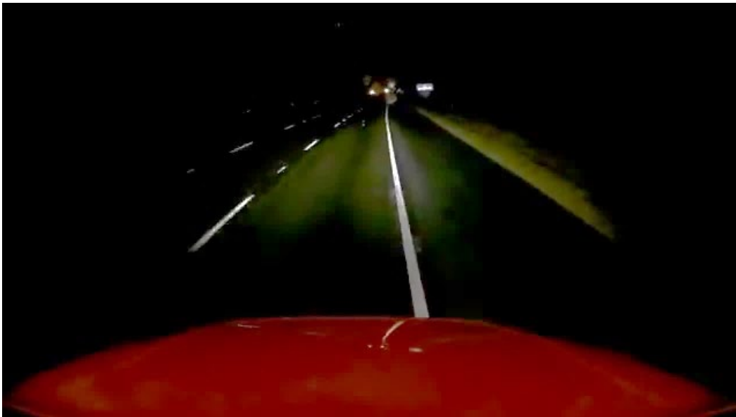
Figure 13. Still-shot from the forward-facing video, showing the combination vehicle crossing the white shoulder line in the 3 minutes leading up to the crash.
