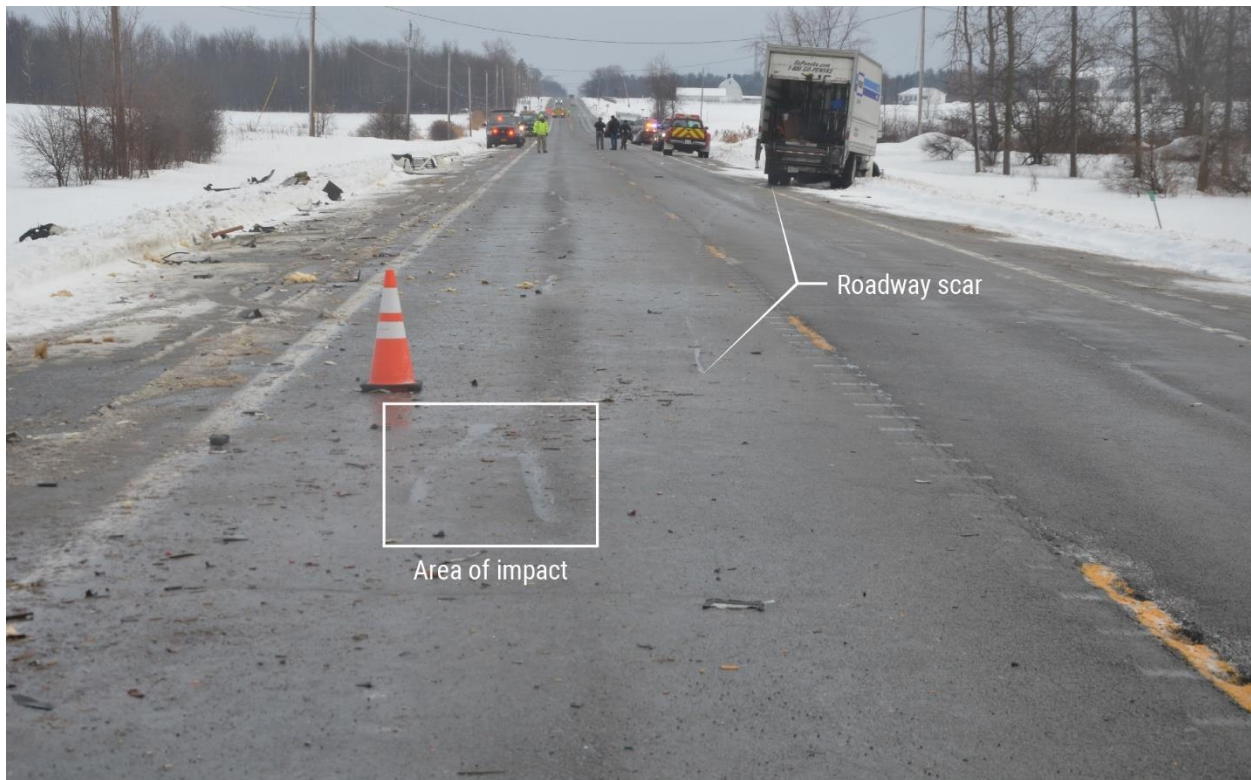
Figure 3. Eastbound SR-37 showing area of impact and roadway scar extending to truck's damaged left front wheel assembly. (Source: New York State Police; annotated by National Transportation Safety Board)
