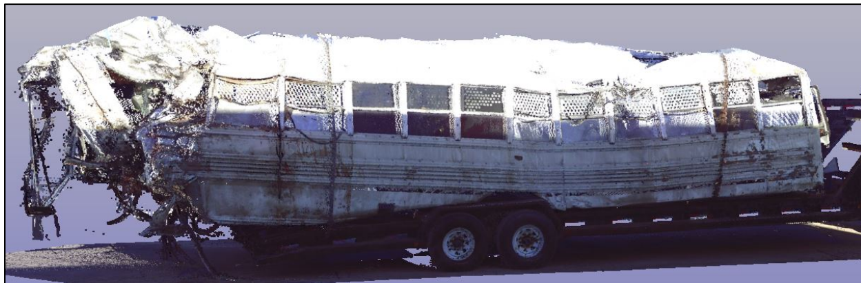
Figure 2. Three-dimensional scan of the left side of the bus involved in the January 14 crash in Penwell, Texas.
