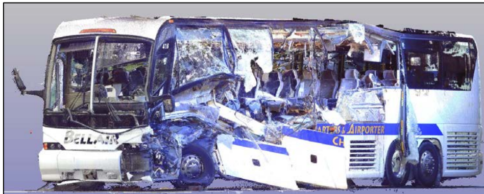
Figure 2: Linked 3D laser scans depicting the damaged left side of the motorcoach.
