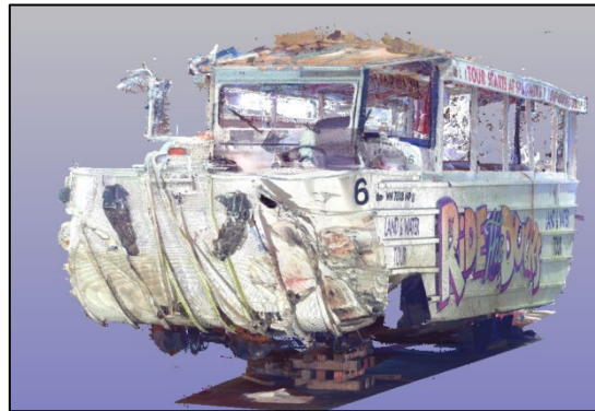
Figure 1: Linked 3D laser scans depicting frontal damage on the accident DUKW vehicle.
