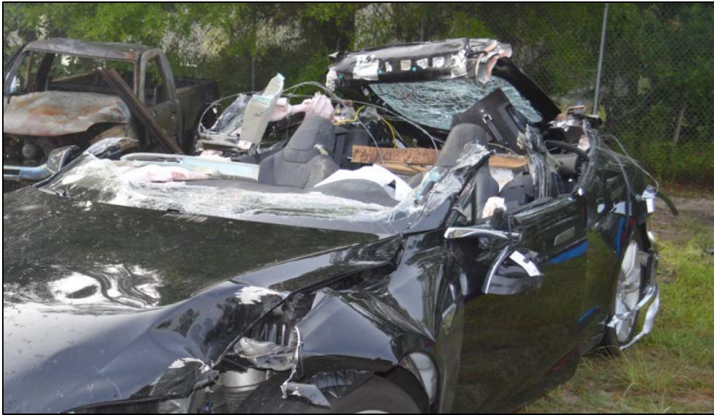
Figure 3. Passenger car damage from impact with semitrailer. (Source: Florida Highway Patrol.)
