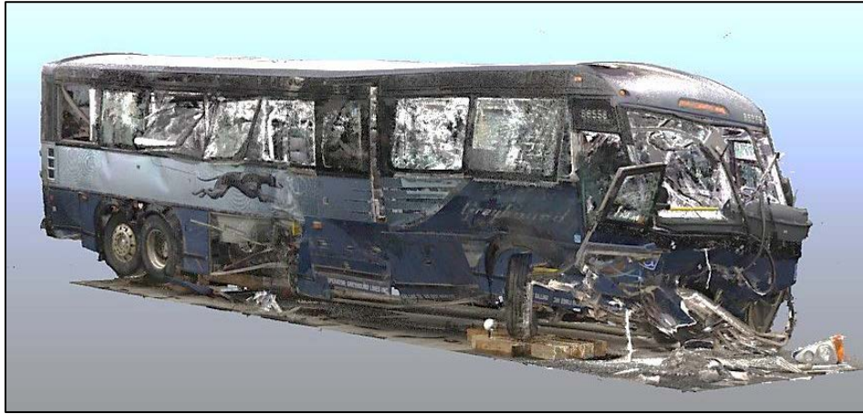
Figure 2. 3D scan image of damaged MCI motorcoach.
