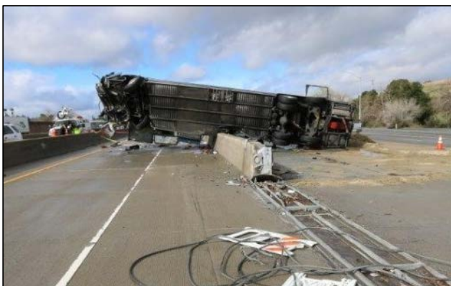
Figure 1. Final rest position of bus and remains of REACT 350 crash attenuator base (left); diagram of exemplar REACT 350 crash attenuator (right). Note: The retroreflective sheeting shown on the first barrel had been damaged and was not present at the time of the crash.
