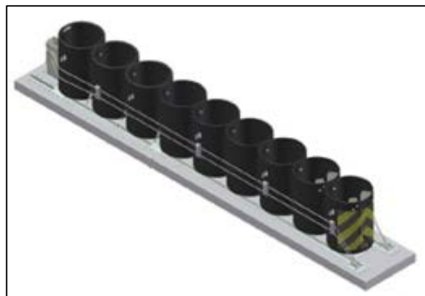
Figure 1. Final rest position of bus and remains of REACT 350 crash attenuator base (left); diagram of exemplar REACT 350 crash attenuator (right). Note: The retroreflective sheeting shown on the first barrel had been damaged and was not present at the time of the crash.
