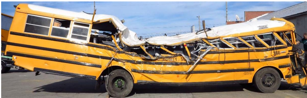
Figure 1. Right side view of school bus showing impact damage.
