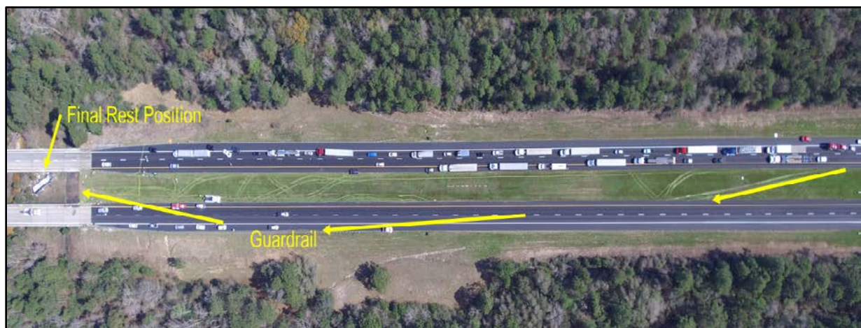
Figure 1. Overhead photo of scene postcrash, showing path and final rest position of motorcoach (yellow arrows).
