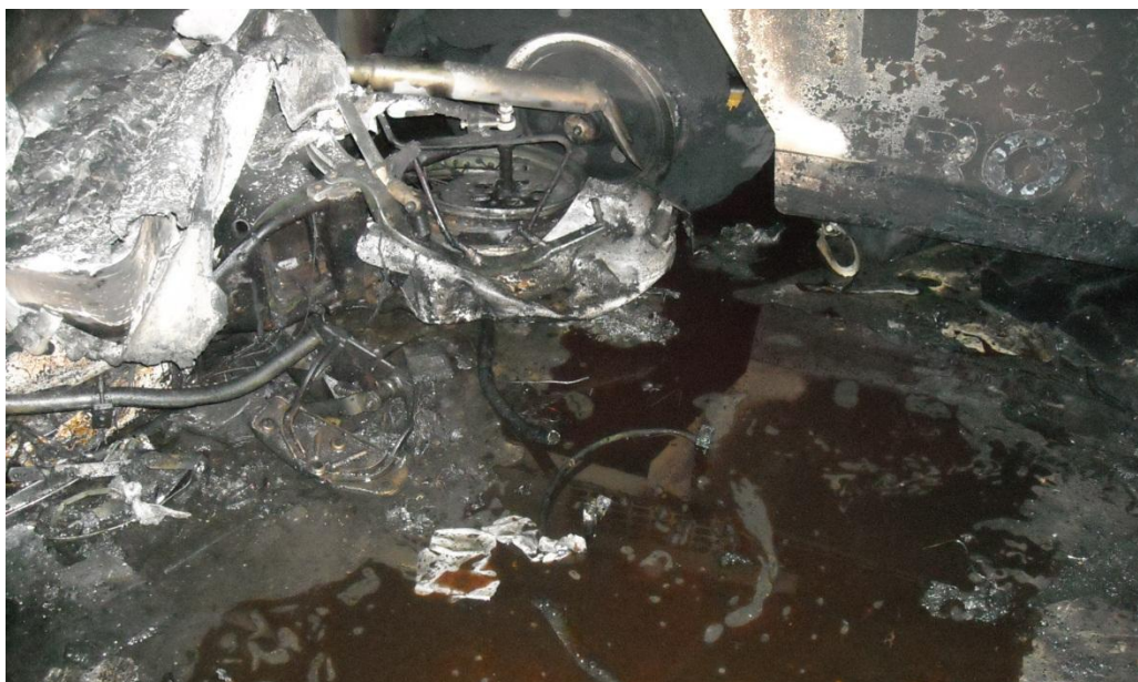
Cargo remains of Harley Davidson motorcycle and pool of oil on deck. (Photo by US Coast Guard)
