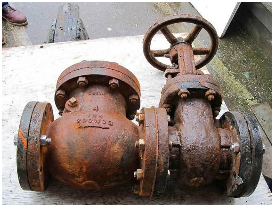
Check (left) and discharge valves from Dry Dock #3. (Photo by Bowditch Marine, Inc.)
