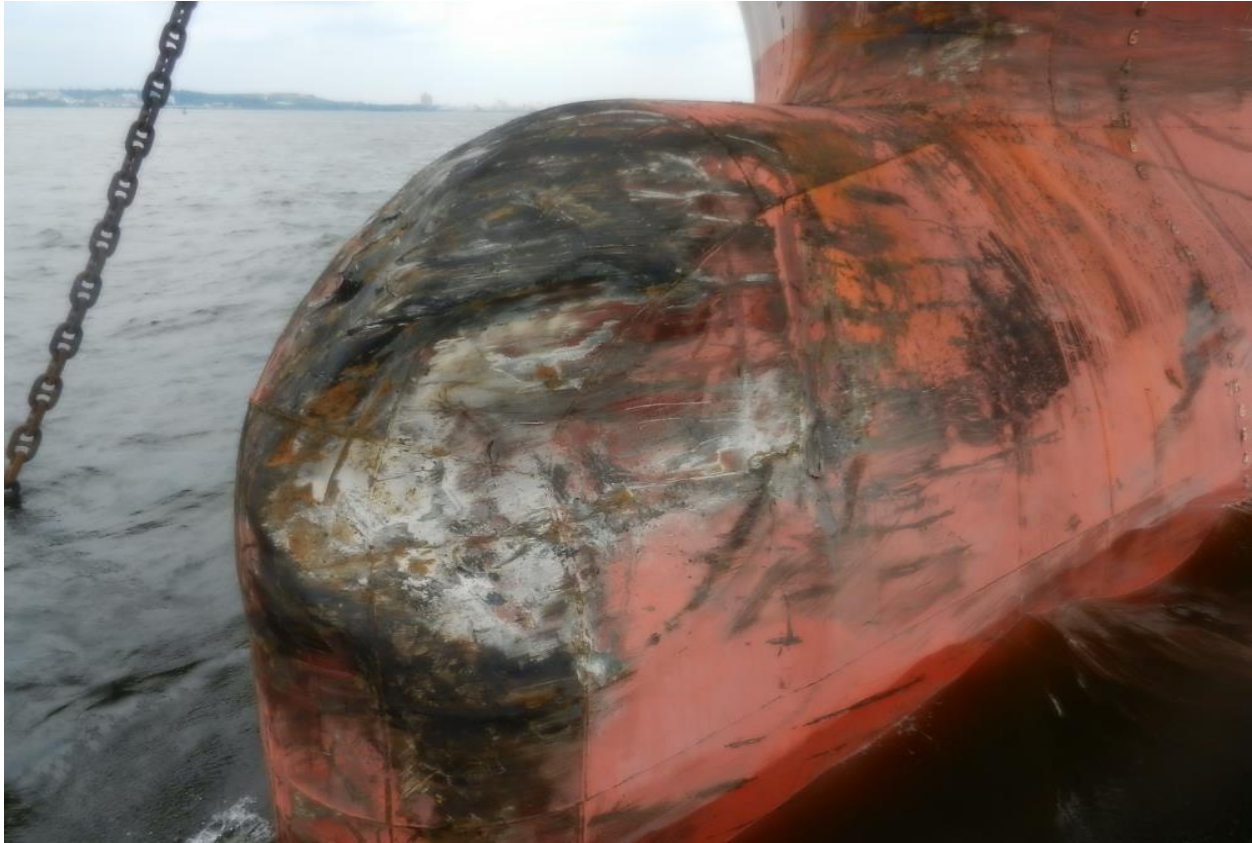
The damaged bulbous bow of the Wawasan Ruby after the allision. (Photo by the Coast Guard)
