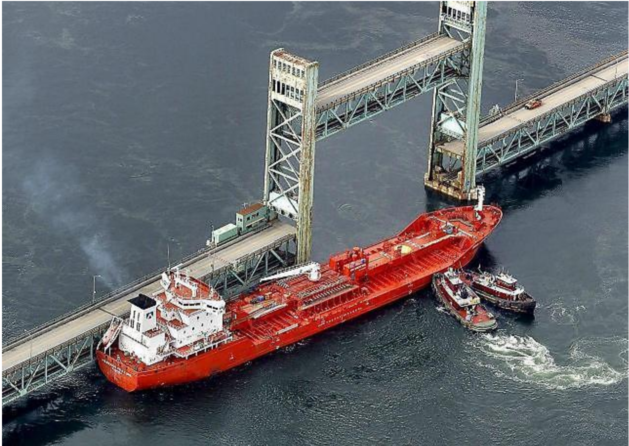
The Harbour Feature pressed against the Sarah Mildred Long Bridge after the allision. Two responding towing vessels, the Mary M. Coppedge and the Drum Point , can be seen on the ship's forward starboard side. (Photo by the Coast Guard)
