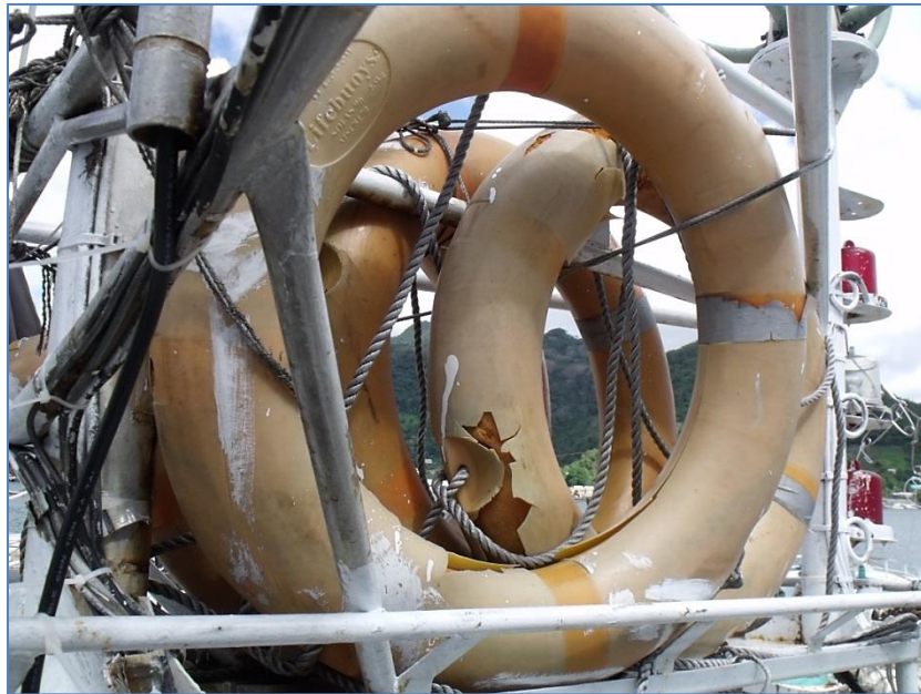
Faded and deteriorated liferings aboard the SeaHawk No. 18 . (Photo by the Coast Guard)
