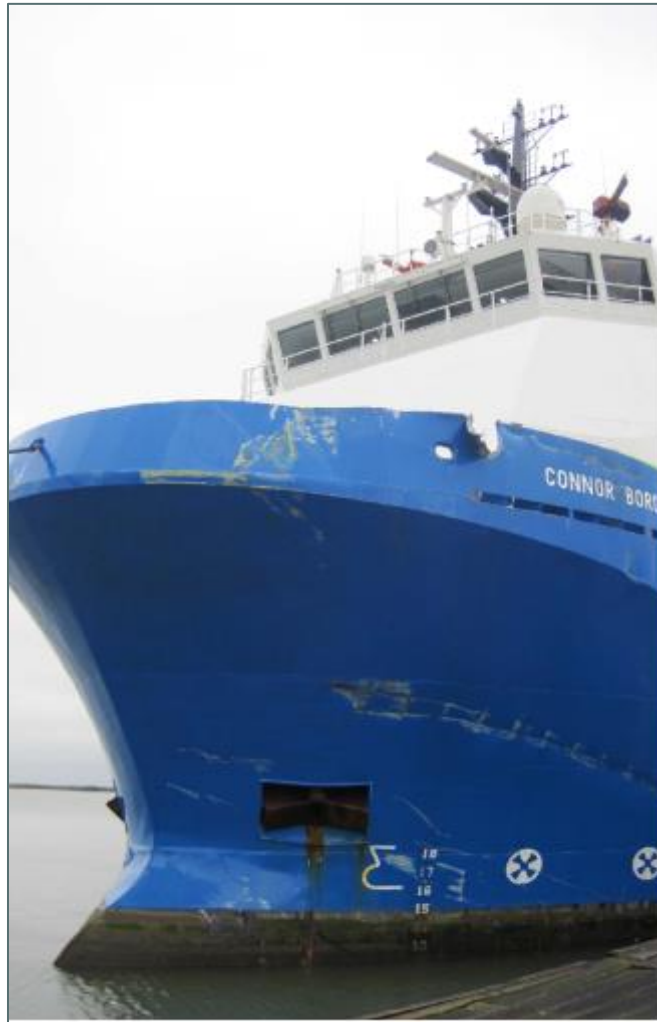
The damage to the Connor Bordelon resulting from its allision with the unmanned platform. The damage included hull scrape marks and a ripped bulwark near the vessel's name. The vessel also sustained damage below the waterline resulting in flooding. (Photo by the Coast Guard)
