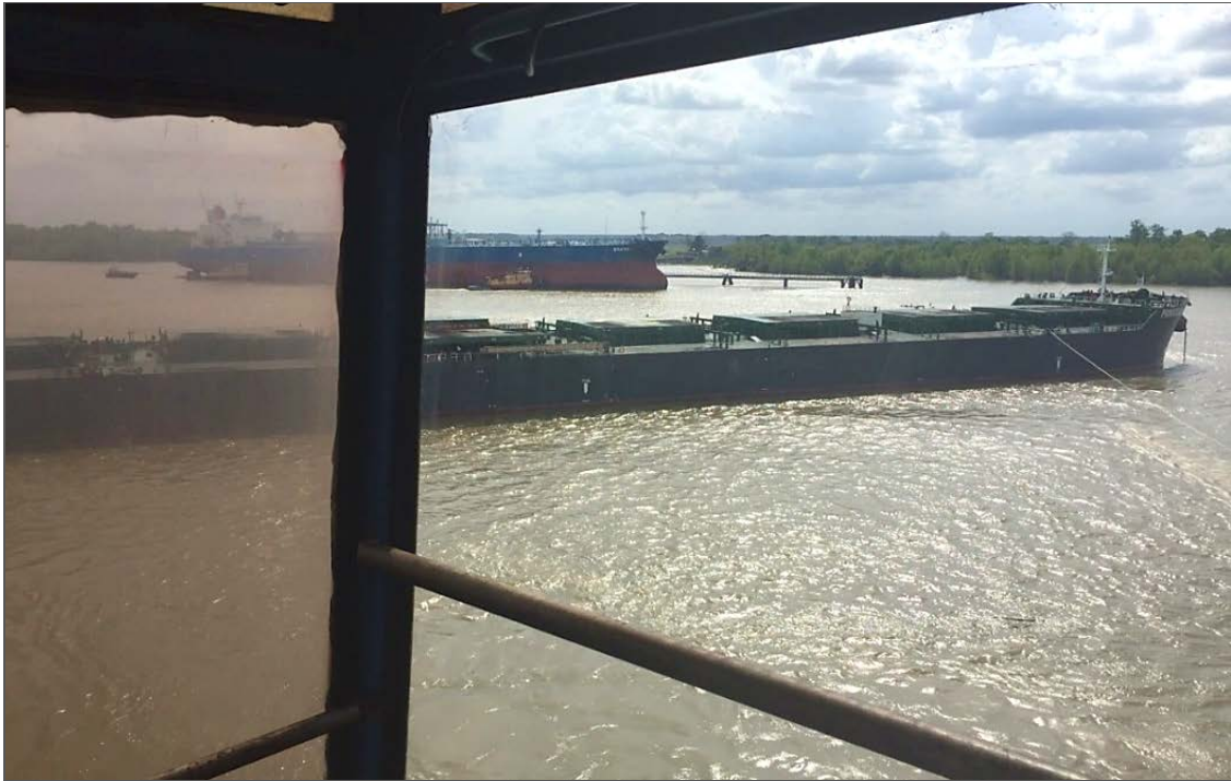
Photo taken by a crane operator at the Convent Marine Terminal, showing the Privocean drifting across the river. A spring line is visible and still connected to the starboard bow of the vessel. In the background, tanker Bravo can be seen moored at the Ergon-St. James Terminal.
