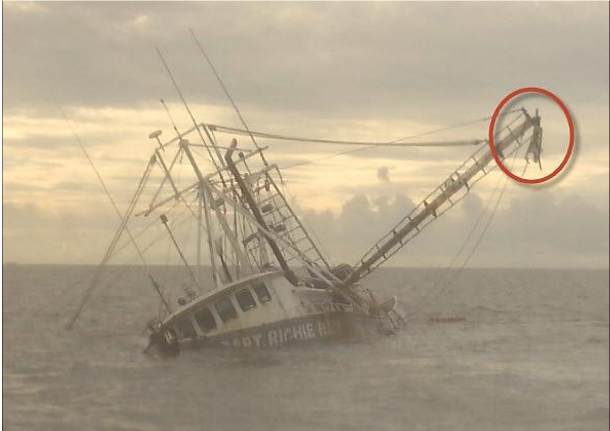
Partially sunken Capt Richie Rich resting on mud in 10–12 feet of water. The broken port outrigger is overlaid by a red circle. (Photo by US Coast Guard)
