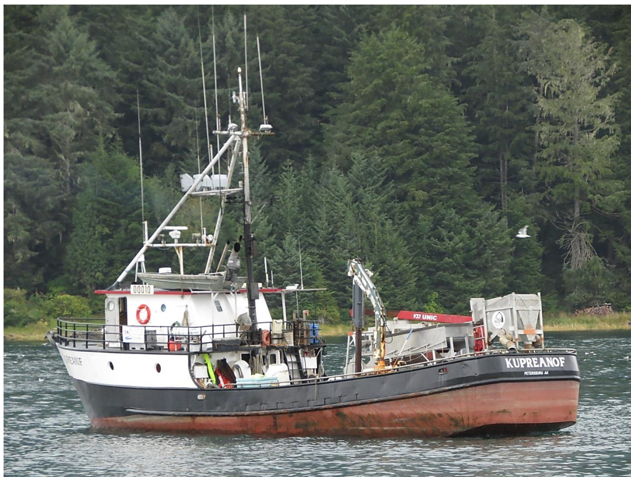
Kupreanof under way prior to the accident. Note equipment lashed to the aft deck that blocked access to the lazarette. (Photo courtesy of Lana Parker)
