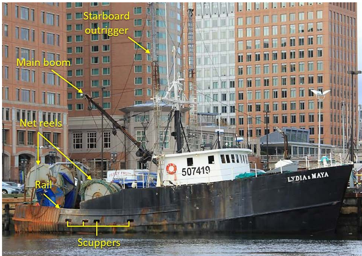
Main boom and net reels on the Lydia & Maya as well as the starboard outrigger, rail, and scuppers. (Photo by Coast Guard)
