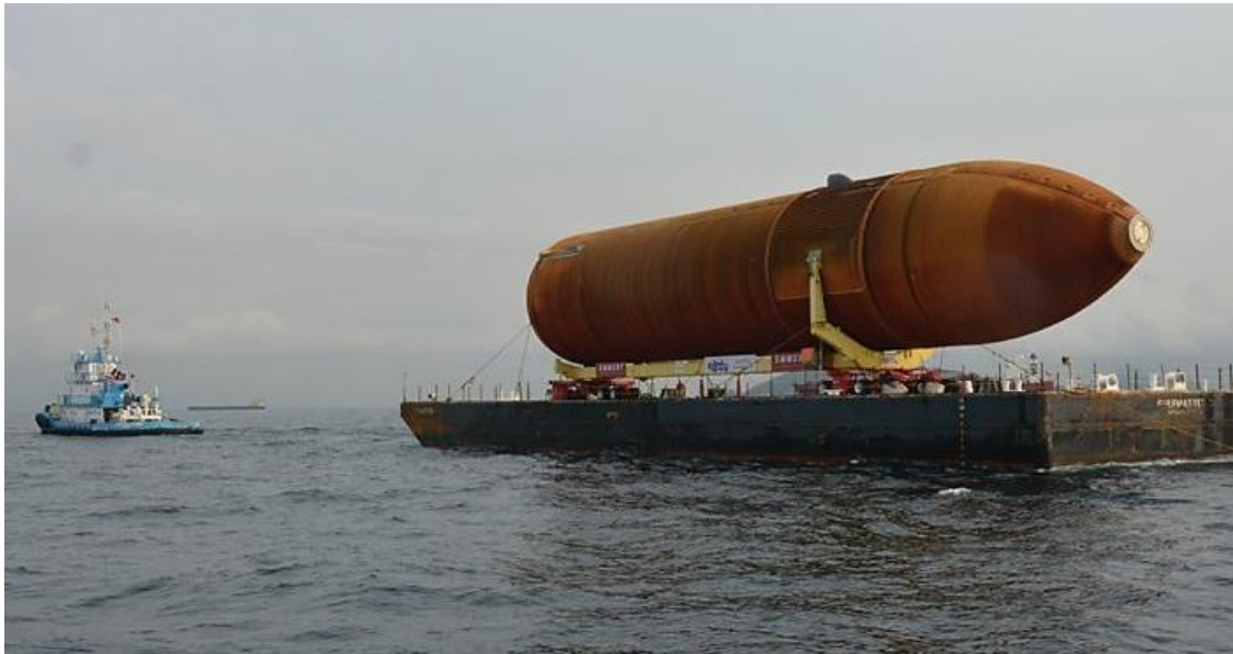
Towing vessel Shannon Dann with space shuttle Endeavour's external fuel tank (ET-94) under tow. (Image by Emmert International)
