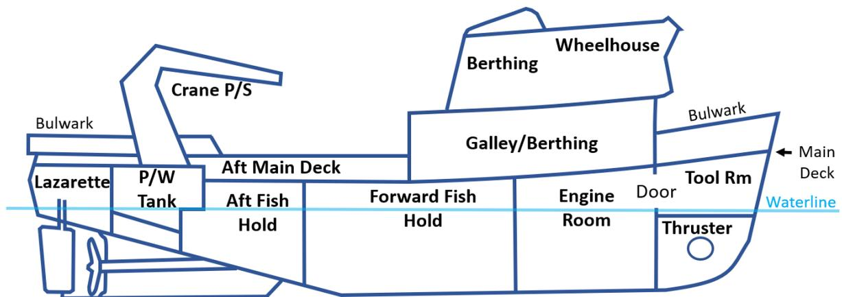
**Simplified side profile of *Ambition*. (Based on original construction general arrangements drawings and captain's description of vessel layout)**
