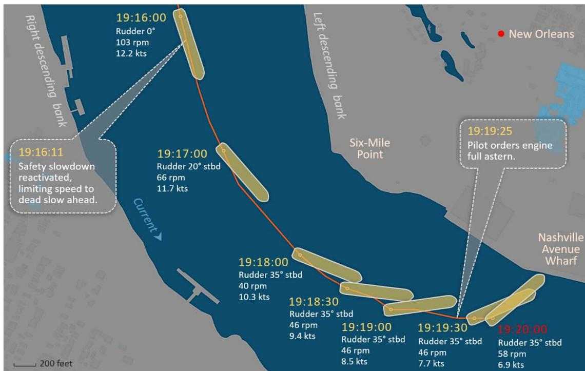
Trackline of *Mia S* over last 4 minutes leading up to accident shows change in vessel's heading and speed over ground following engine slowdown. (Background from Google Maps)
