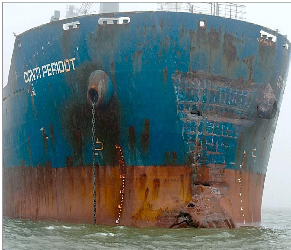
Figure 12. The damaged bow of the Conti Peridot . (Photo by Port of Houston Authority Fire Department)
