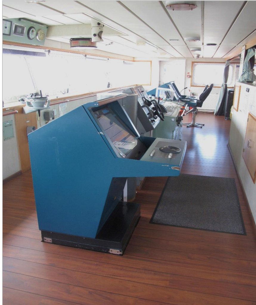
Figure 6. The Carla Maersk navigation bridge, shown from port to starboard. Consoles are equipped with radars, electronic chart display and information system (ECDIS), steering controls, and engine telegraph and communications equipment.
