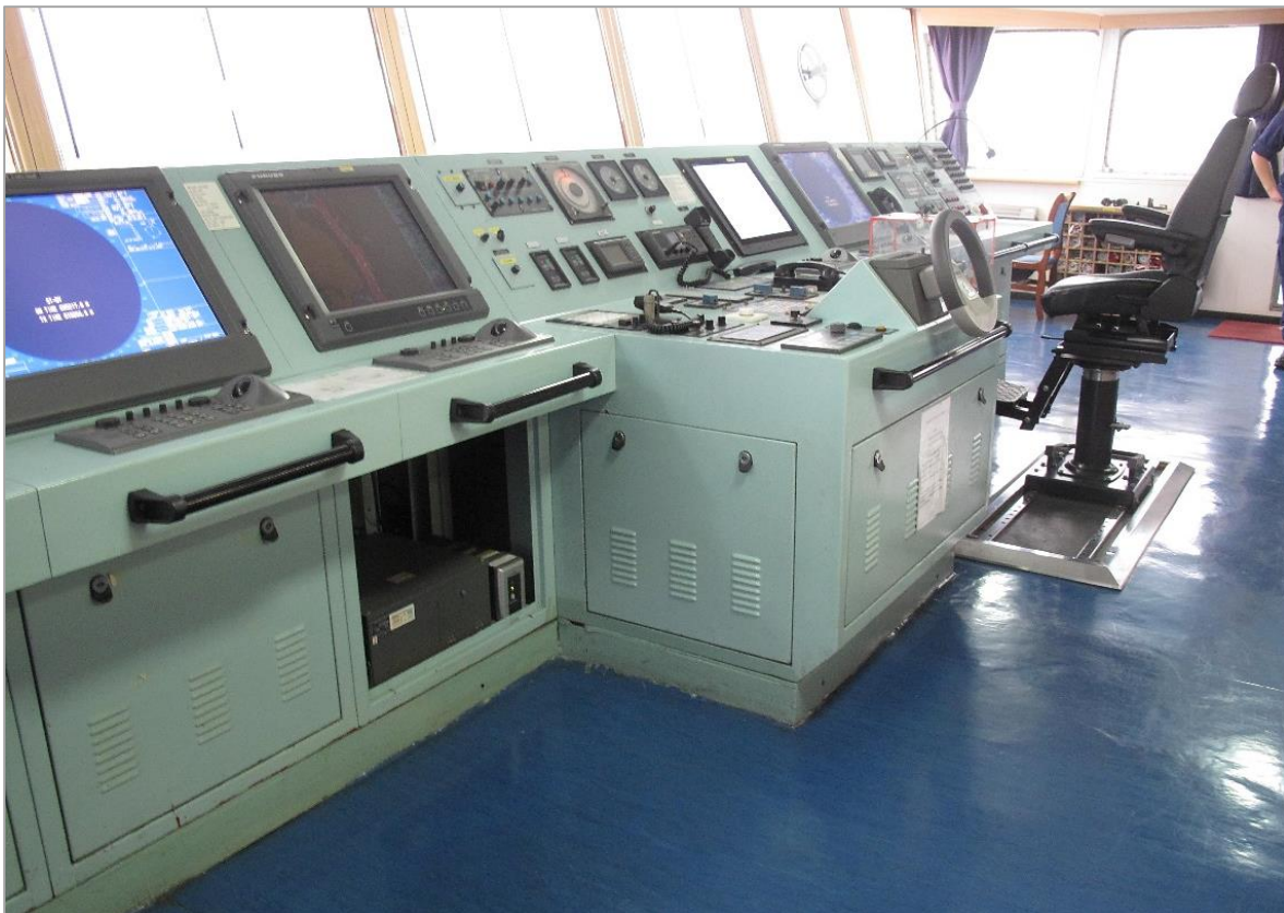
Figure 7. The Conti Peridot navigation bridge, shown from port to starboard. Consoles are equipped with radars, ECDIS, steering controls, and engine telegraph and communications equipment.
