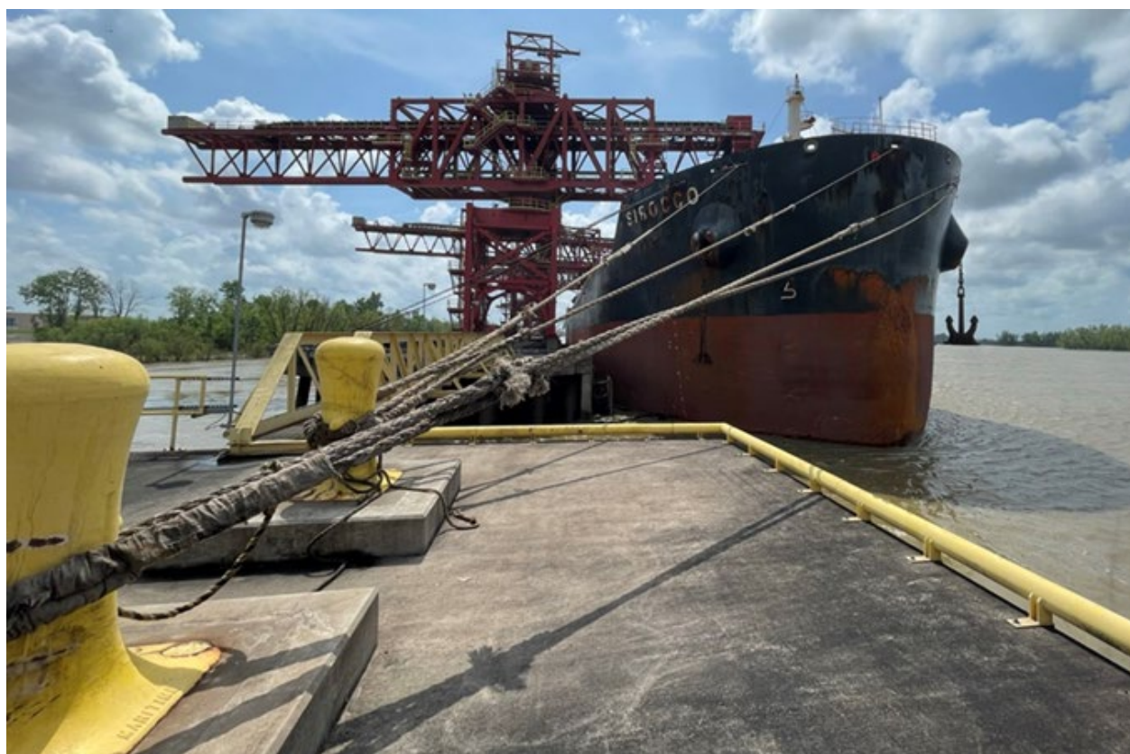
Figure 3. The forward mooring arrangement of the Sirocco at the CMT dock at 1227 on March 26, 2023. (Source: Oldendorff port captain)
