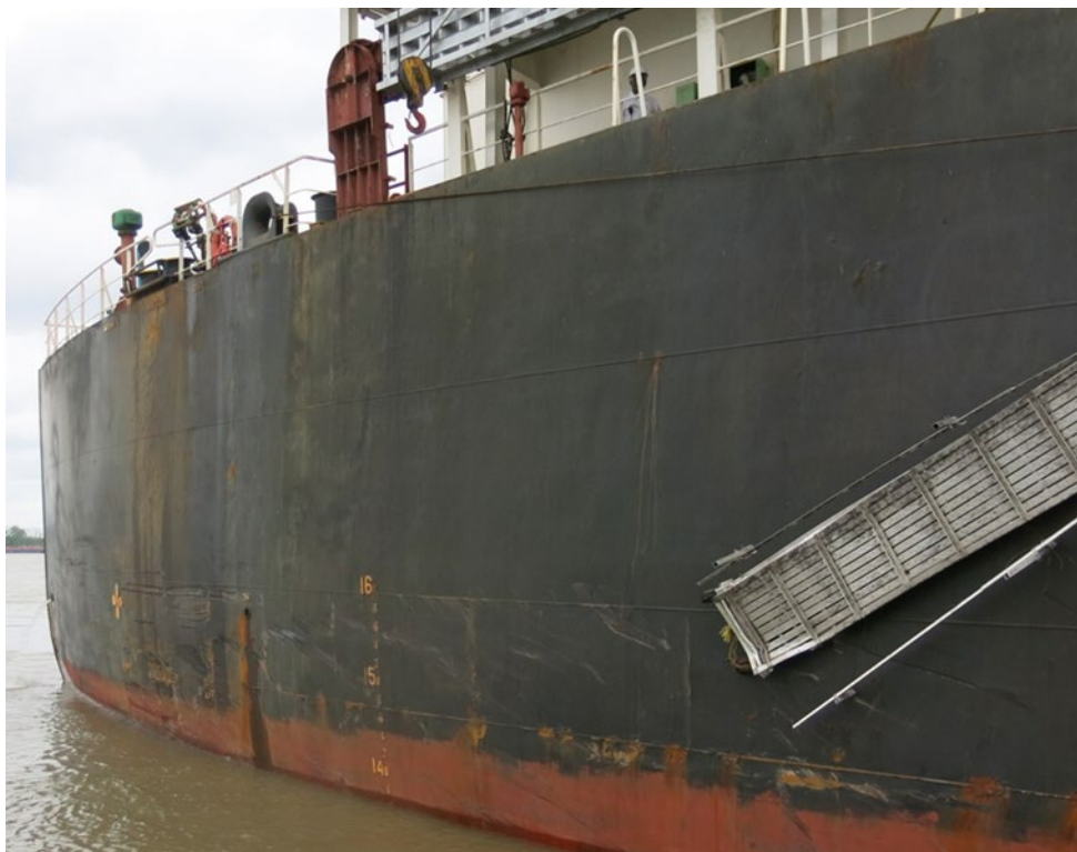
Figure 8. The Sirocco 's damaged starboard-side accommodation ladder.
