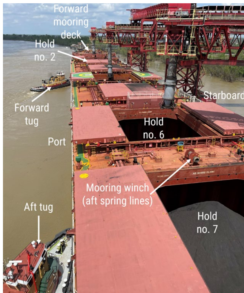
Figure 5. The two tugs on the Sirocco 's port side on March 26 at 1314. (Background source: Oldendorff port captain)
