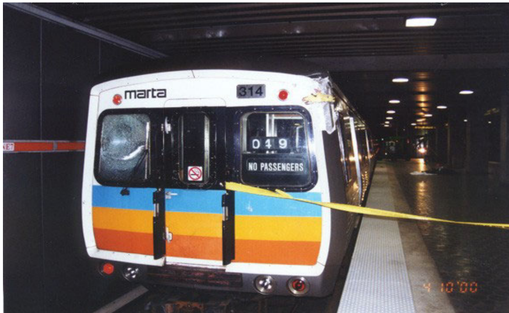
Figure 3. Lead car of April 10, 2000, Lenox Station accident train; window damaged by contact with work boom of self-propelled lift.
