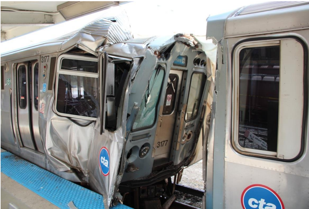
Figure 2: Crumpled lead car of passenger train 110 and minimally damaged striking car.
