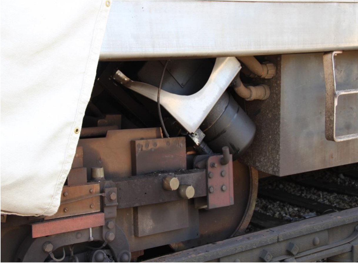
Figure 3: Derailed wheel and axle of the lead truck on the lead car.
