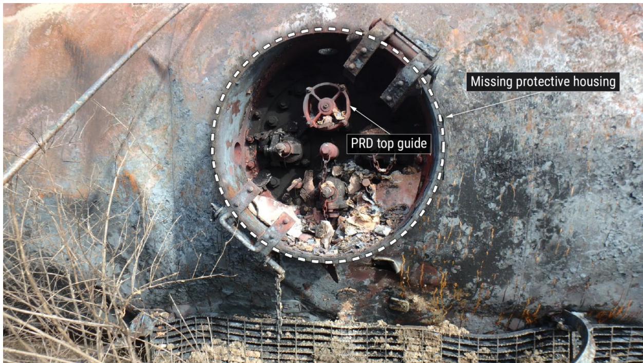
Figure 21. Tank car OCPX80235's protective housing with the aluminum cover missing.
