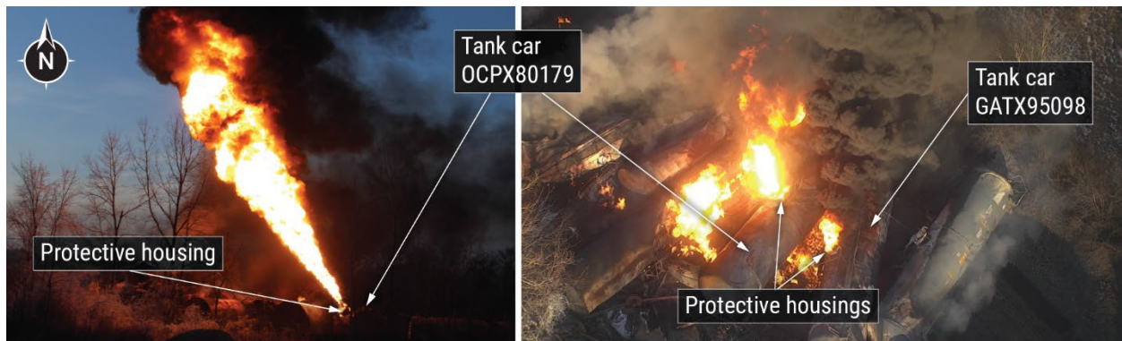
Figure 8. PRDs venting material energetically (left) and more typically (right).
