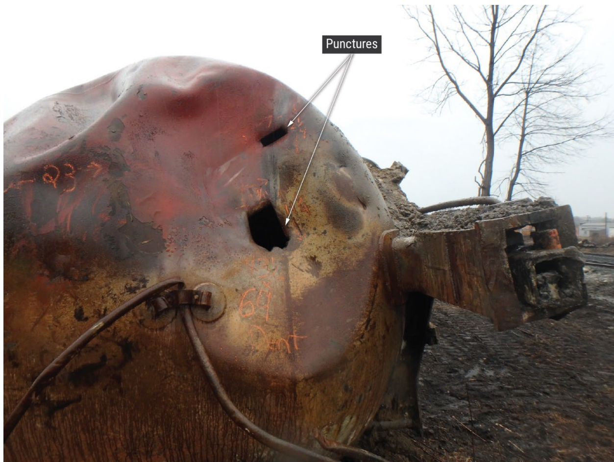
Figure 20. Leading A-end head punctures on tank car UTLX205907.
