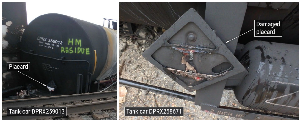
Figure 26. Postderailment photographs of placards exposed to heat.
