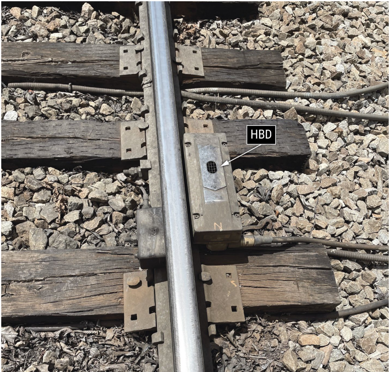
Figure 13. Example of a Progress Rail Micro HBD.
