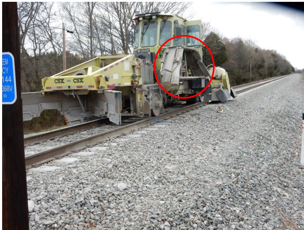
Figure. Photograph of the ballast regulator at the accident site. The area where the operator was trapped is circled. (Photograph provided by the Federal Railroad Administration.)
