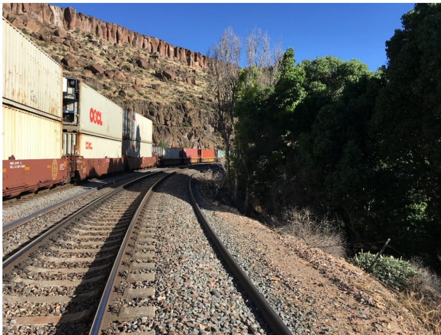
Figure 2. Viewpoint of the approaching intermodal train entering the 8° curve just before the point of collision.
