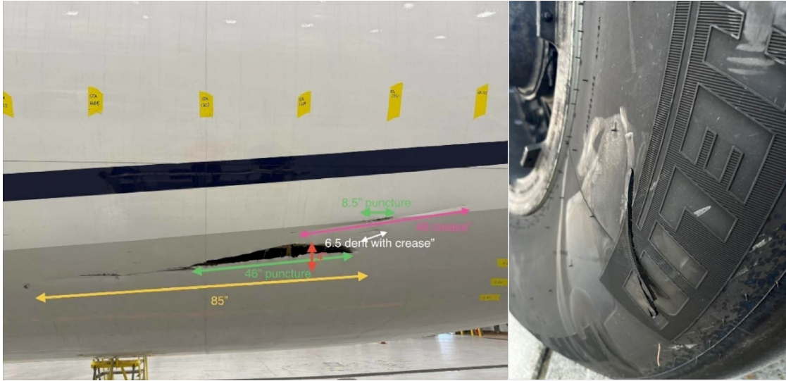
Figure 7. Right photo shows the left lower aft fuselage damage, and the left photo shows the damage to the #1 left MLG tire. (Source: United Airlines)
