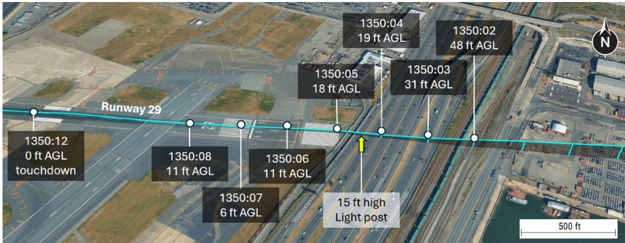
Figure 3. Google Earth image showing the New Jersey turnpike, light post and approach end of runway 29. Note: the turnpike is 5 ft higher than the runway and altitude is depicted as height above ground, so the airplane descended a total of 6 ft between 1350:04 and 1350:05.
