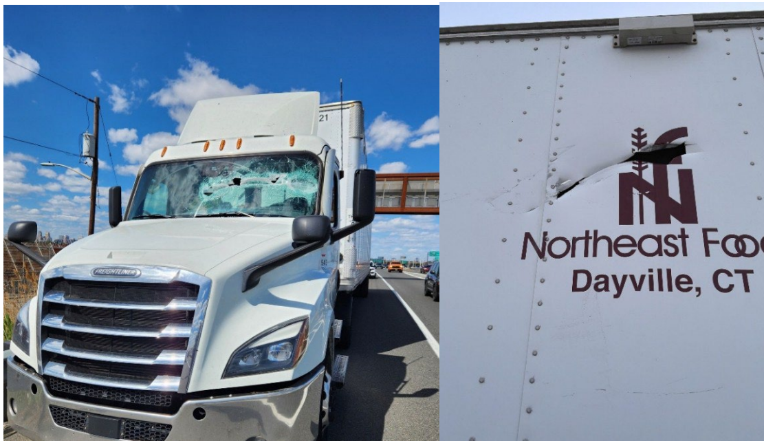
Figure 8. Left photo shows the damage to the tractor cab's windshield, and the right photo is front face of the trailer. (Source: left photo Port Authority, right photo NTSB)
