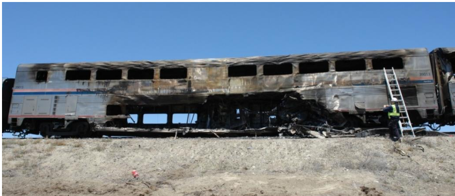
Figure 5. Photograph of crew sleeper railcar 39013, with front of railcar at left, showing where accident truck-tractor penetrated lower level and ensuing fire engulfed railcar.
