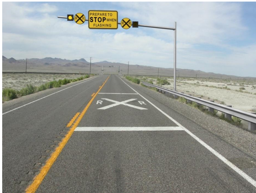
Figure 24. Depiction of proposed active advance warning sign to be constructed on approach to Miriam, Nevada, grade crossing.
