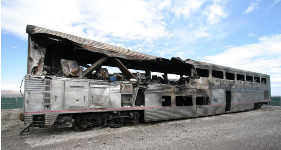
Figure 6. Photograph of first coach railcar 34033 at impound lot, with front of railcar at left, showing extent of damage caused by collision with first side-dump trailer and fire damage throughout railcar.
