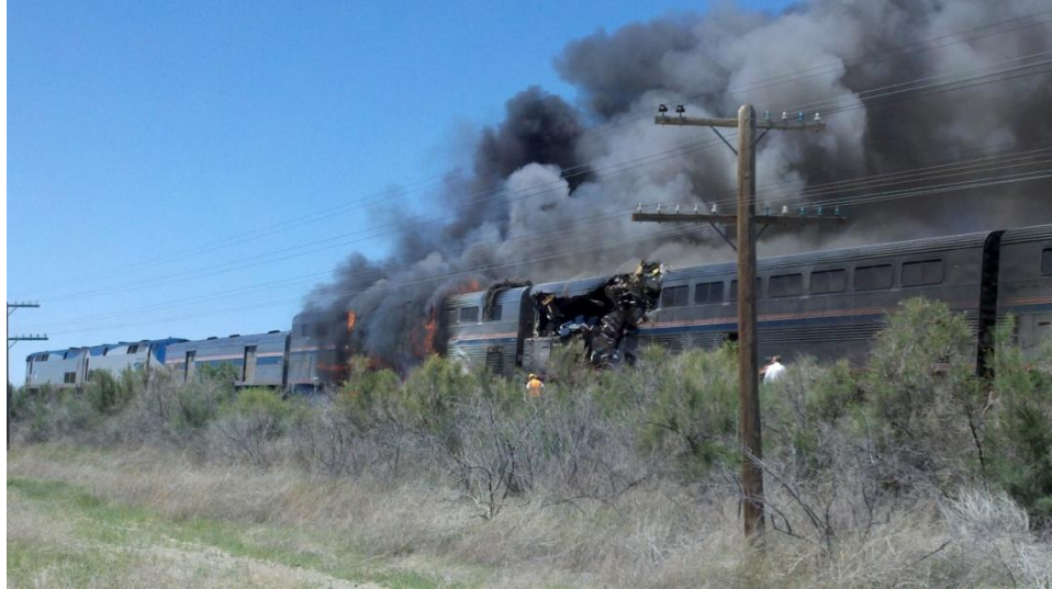
Figure 3. From left to right, photograph showing two locomotives, baggage railcar, burning crew sleeper railcar, first coach railcar with large opening where penetrated by first side-dump trailer, and front of second coach railcar. (Courtesy of rail passenger)
