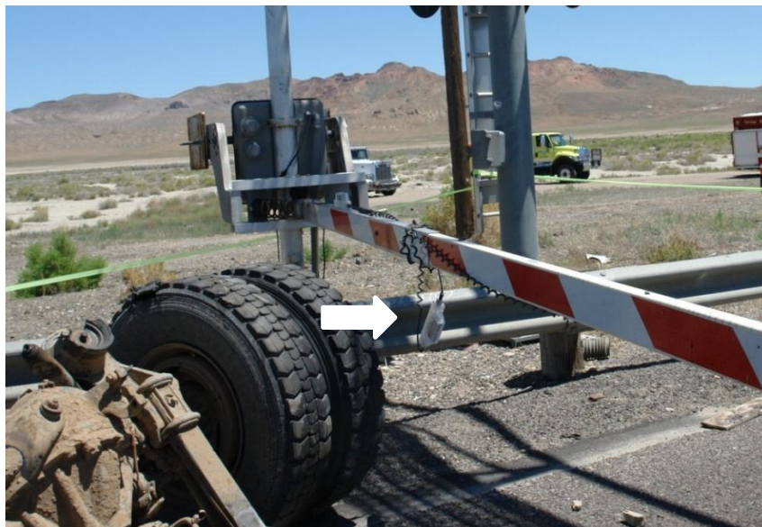
Figure 18. Photograph showing detached center light of crossing gate arm hanging from its power cord and fourth axle from accident truck at bottom left. (Courtesy of Nevada Highway Patrol)
