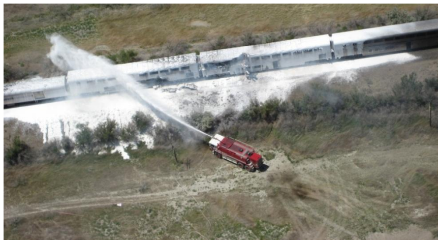
Figure 4. Aerial photograph showing all-wheel-drive foam pumper truck extinguishing fire on Amtrak train. (Courtesy of Nevada Highway Patrol)
