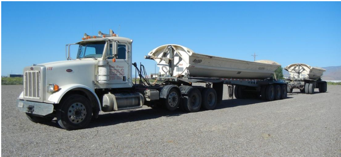
Figure 10. Photograph of exemplar Peterbilt truck-tractor in combination with two SmithCo side-dump trailers.
