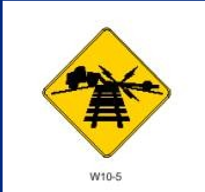
Low-ground clearance warning sign
