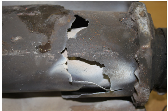
Figure 2. Fractured exhaust muffler from a Hefty Polar Cub airplane (left) and a close-up photograph of the fracture in the exhaust muffler (right).
