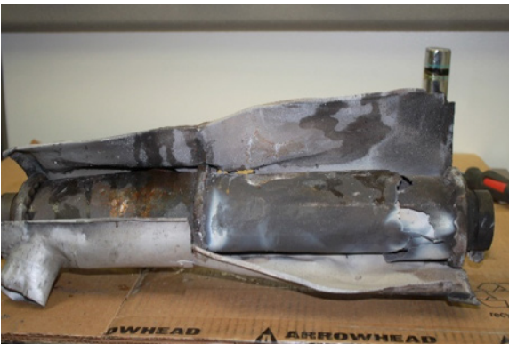
Figure 2. Fractured exhaust muffler from a Hefty Polar Cub airplane (left) and a close-up photograph of the fracture in the exhaust muffler (right).
