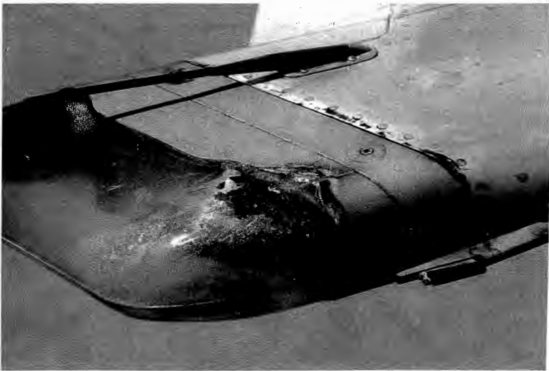
Figures 1a and 1b.--Lightning damage to right wing tip.
