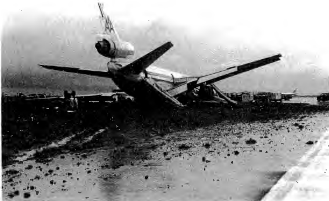
Figure 3b.--Tire marks on high speed taxiway 3S, and trenches in the soil leading to the final resting position of the airplane.
