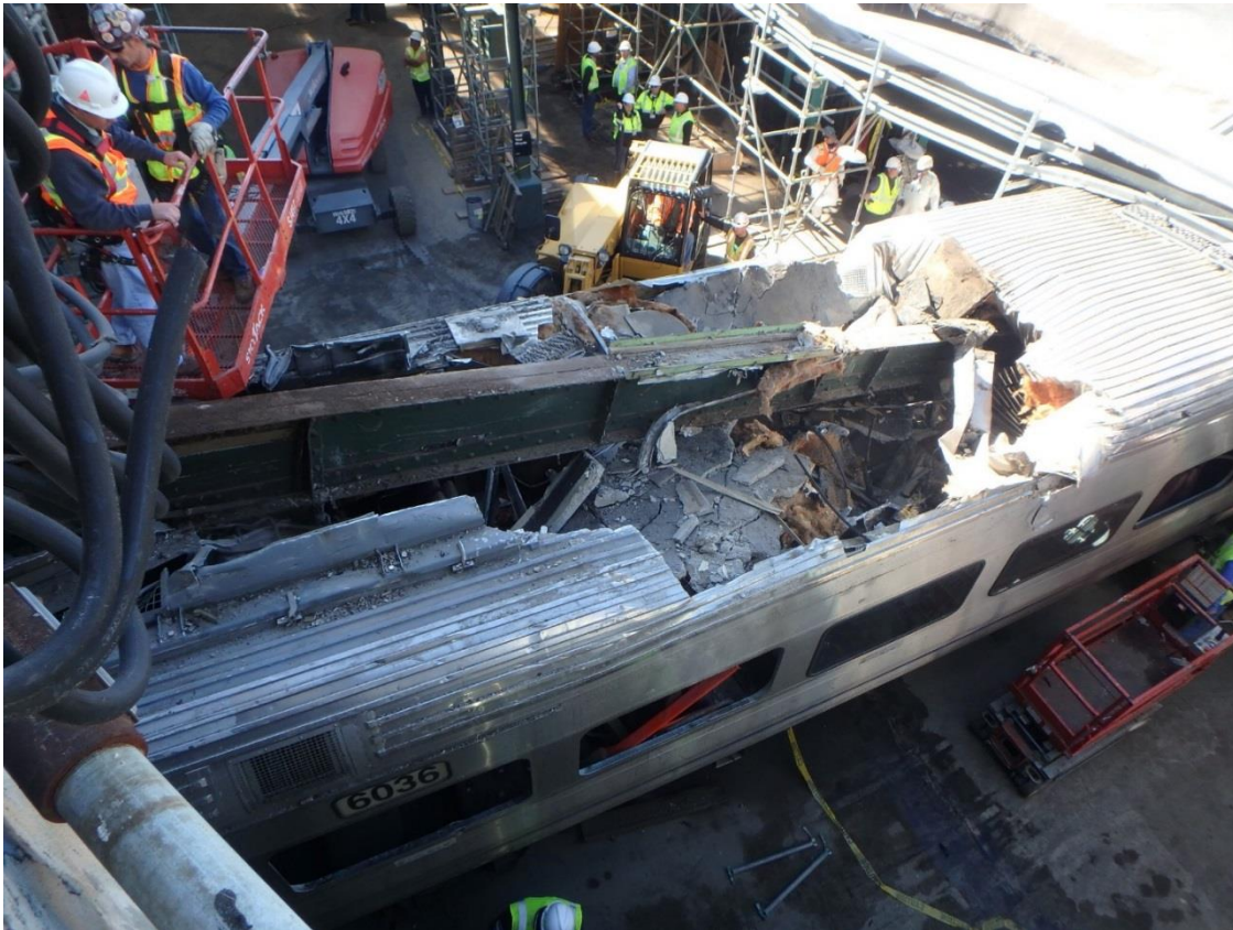
Figure 1. Damaged controlling cab car.
