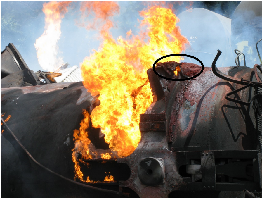
Figure 2: Bulge in the tank shell of the burning tank car. (Photograph courtesy of CSX.)
